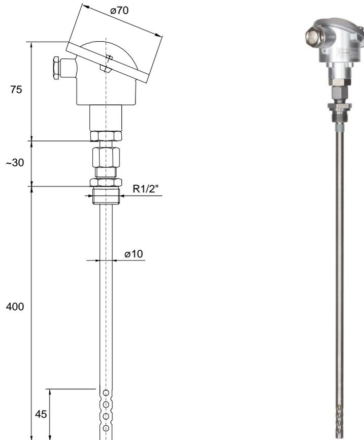
Screw-in resistance thermometer with terminal head and movable screw joint, measuring resistance 1x PT100 fixed built-in.
